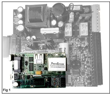
Top view of multi-protocol card installed on ES749 mother board
