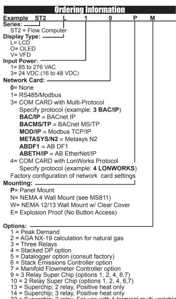
22 = Superchip; 2 relay, For use with 4 terminal multi-variable vortex meters
