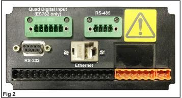
Rear view of ES749 case. Communication ports are available for RS-485 and Ethernet
